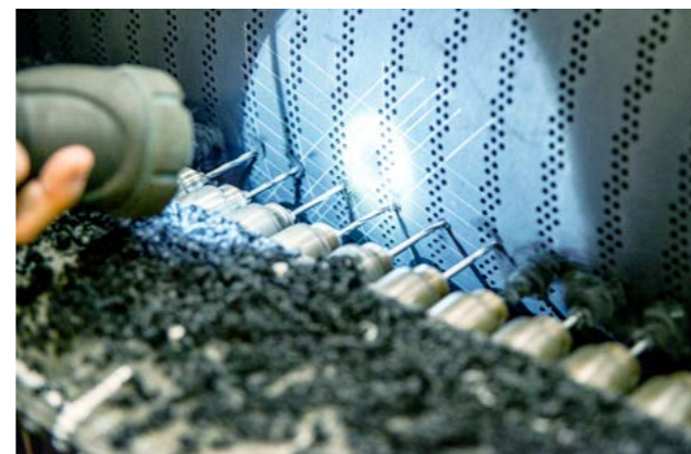
Roll cover drilling process
