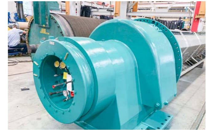
Refurbished suction box
