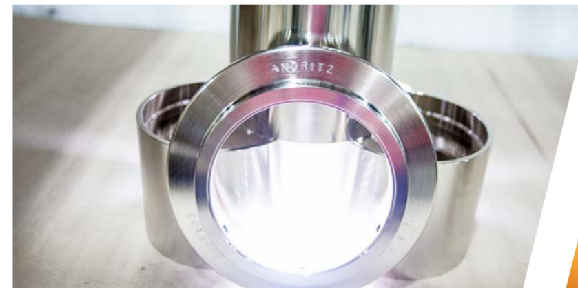
Custom engineered spreader roll components after CNC machining and nickel plating
