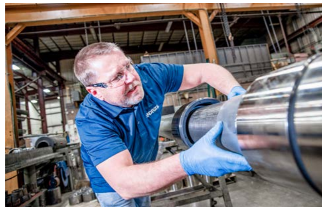
All metal spreader roll during spool assembly
