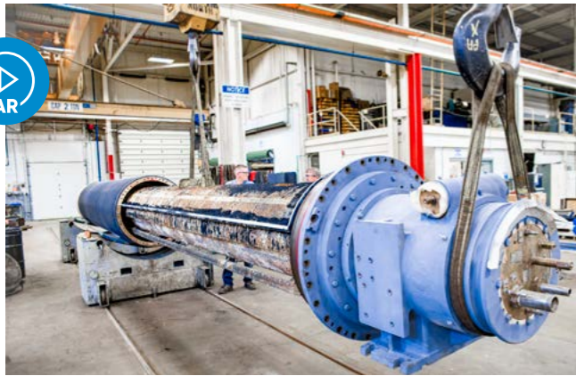
Suction box being removed from suction roll
