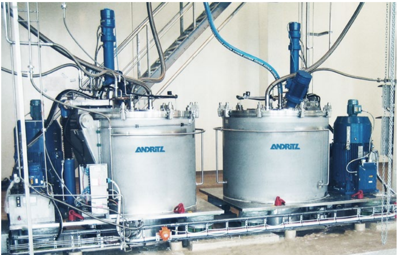
Typical installation of two vertical centrifuges VZU 1250
