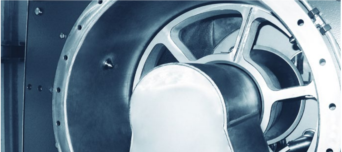
Solids discharge outlet
